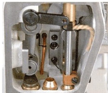
Needle bar drive with lubrication by oil wick and vacuum suction
